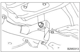
5) Remove center exhaust pipe and rear catalytic converter assembly from hanger bracket.
