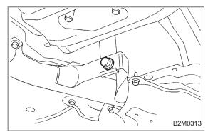
4) Tighten bolt which holds center exhaust pipe to hanger bracket.
