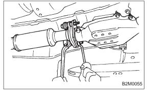
3) Separate center exhaust pipe and rear catalytic converter assembly from rear exhaust pipe.
