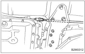
5) Connect rear oxygen sensor connector. (Except California 2200 cc model)
