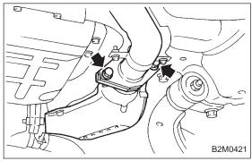
4) Separate center exhaust pipe and rear catalytic converter assembly from front catalytic converter.
