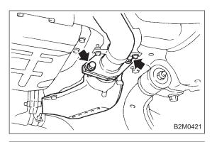
2) Install center exhaust pipe to front catalytic converter.
