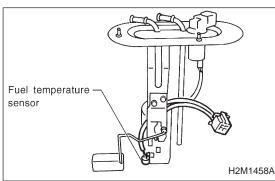
8) Remove fuel temperature sensor from fuel pump assembly.
