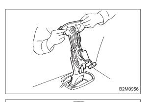
5) Take off fuel pump assembly from fuel tank.
