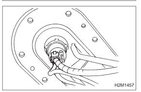
7) Disconnect connector from fuel pump.
