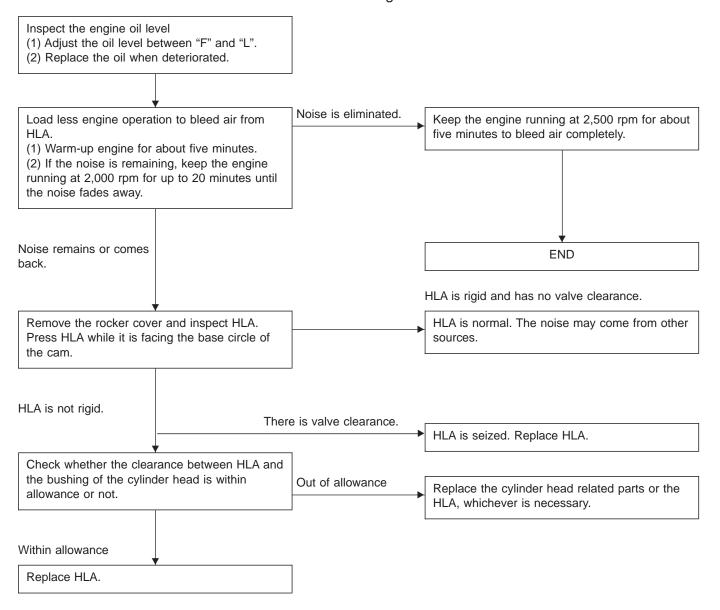
If noise still exists, conduct diagnostics procedures in accordance with the following table.
