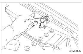
8) Connect ground cable to battery terminal.
