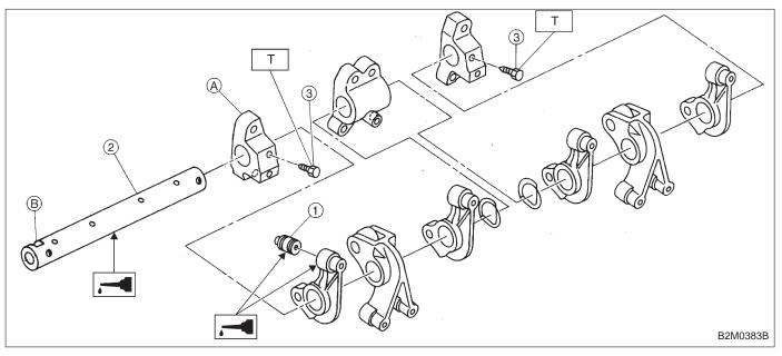
Tightening torque: N⋅m (kg-m, ft-lb) T: 5±1 (0.5±0.1, 3.6±0.7)
