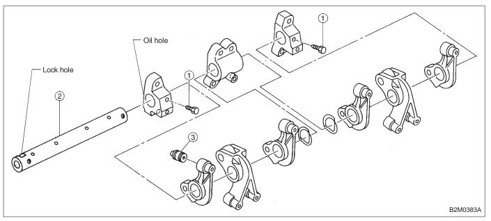
1) Remove bolts which secure rocker shaft.
