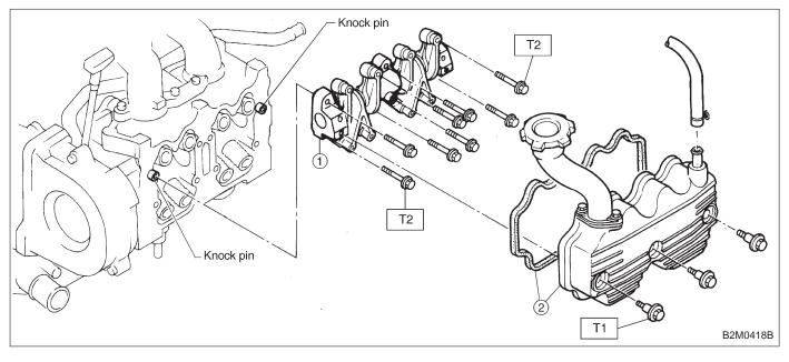
Tightening torque: N·m (kg-m, ft-lb) T1: 5±1 (0.5±0.1, 3.6±0.7) T2: 12±1 (1.2±0.1, 8.7±0.7)
