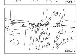
6) Connect rear oxygen sensor connector. (Except California 2200 cc model)
