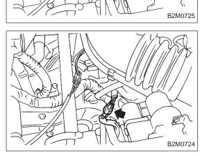
9) Connect front oxygen sensor connector.
