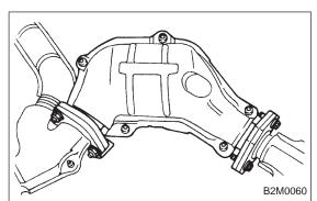
8) Separate front exhaust pipe from front catalytic converter.
