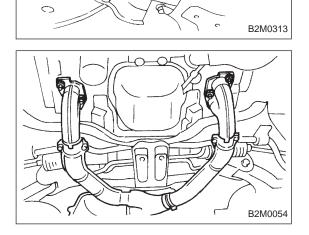
3) Tighten bolts which hold front exhaust pipe onto cylinder heads.
