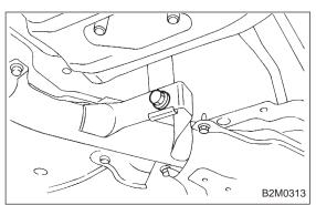
7) Remove front exhaust pipe and center exhaust pipe from hanger bracket.
