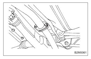
2) Install rear exhaust pipe to muffler.
