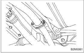
2) Separate rear exhaust pipe from muffler.
