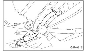
3) Remove rear exhaust pipe bracket from rubber cushion.
