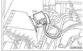
2) Disconnect connector from mass air flow sensor.
