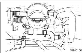
5) Disconnect engine coolant hoses from throttle body.
