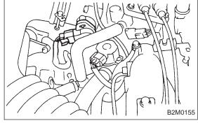
4) Disconnect connector from throttle position sensor.
