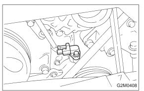
6. Crankshaft Position Sensor A: REMOVAL AND INSTALLATION
