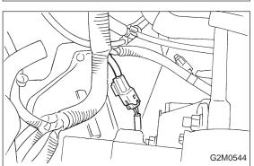
2) Disconnect connector from front oxygen sensor.
