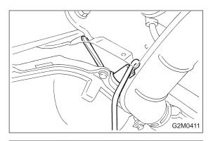
5) Remove front oxygen sensor.
