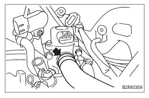
3) Disconnect by-pass hose from idle air control solenoid valve.
