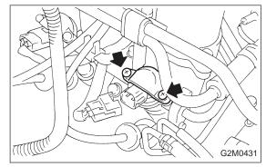
3) Remove fuel injector from fuel pipe assembly.
