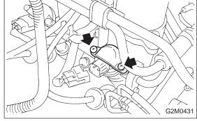
3) Remove fuel injector from fuel pipe assembly.
