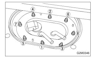
10) After draining fuel, reinstall fuel pump. Tighten nuts in numerical sequence shown in Figure to specified torque.
