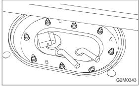
7) Remove nuts which install fuel pump assembly onto fuel tank.
