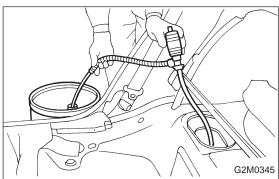
9) Drain fuel from fuel tank by using a hand pump.
