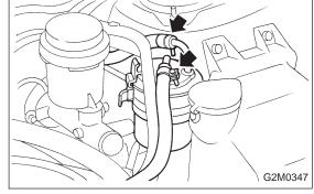
3) Disconnect fuel delivery hoses from fuel filter, and connect fuel pressure gauge.
