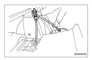
11) On AWD model, after removing fuel sub meter unit, drain fuel from there.
