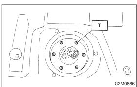
7) Installation is in the reverse order of removal procedure. *Tightening torque: T: 3 — 6 N·m (0.3 — 0.6 kg-m, 2.2 — 4.3 ft-lb)*
