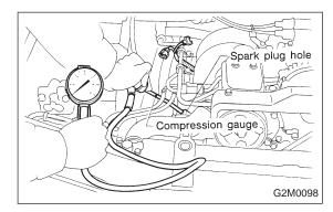
7) Hold the compression gauge tight against the spark plug hole.
