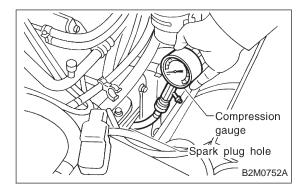
7) Hold the compression gauge tight against the spark plug hole.
