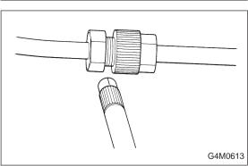
(3) Check the area where the nut joins the tube.
