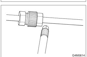
3) Check the area of the sight glass and pressure switch (dual switch), and also check the seams of the receiver drier.
