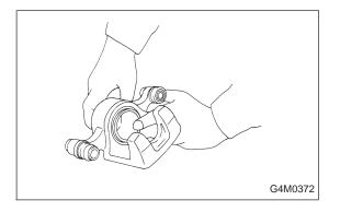
5) Insert piston into cylinder.
