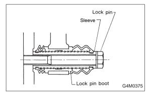
5) Apply a coat of specified grease to boot and fit in groove on ends of cylinder and piston.
