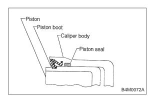
6) Position boot in grooves on cylinder and piston.
