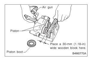
4) Gradually supply compressed air via caliper body brake hose to force piston out.
