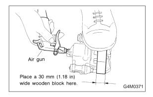
2) Gradually supply compressed air via caliper body brake hose to force piston out.
