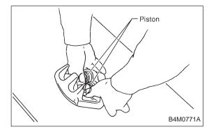
4) Insert piston into cylinder.
