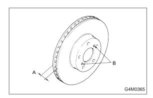
5) Remove disc rotor from hub.
