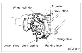
7) Remove shoes one by one from back plate with adjuster.
