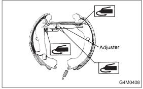
3) Apply grease to adjusting screw and both ends of adjuster.
