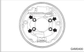
6) Remove the bolts installing back plate, and then, remove brake assembly.
