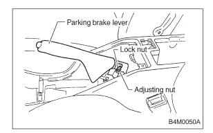
6) Adjust parking brake lever by turning adjusting nut until parking brake lever stroke is set at 7 to 8 notches with operating force of 196 N (20 kg, 44 lb).
