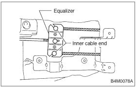
7) Remove inner cable end from equalizer.
