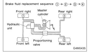
5) Install one end of a vinyl tube onto the air bleeder of and insert the other end of the tube into a container to collect the brake fluid.
