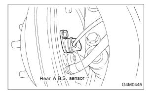
2) Temporarily install rear ABS sensor on back plate.
