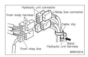
2) Secure relay box connector to connector bracket.
