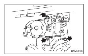
6) Remove nuts and bolt which secure hydraulic unit bracket, and remove hydraulic unit from engine compartment.
