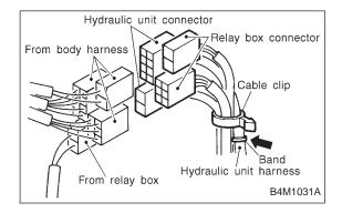
4) Secure hydraulic unit connector to connector bracket.
