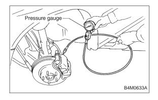
3) Connect two pressure gauges to the FL and FR caliper bodies.
