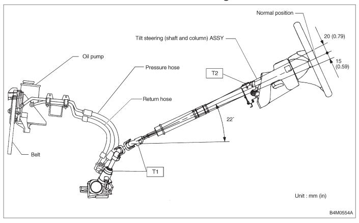
Tightening torque: N·m (kg-m, ft-lb) T1: 24±3 (2.4±0.3, 17.4±2.2) T2: 25±5 (2.5±0.5, 18.1±3.6)
