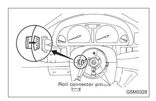
6) Align center of roll connector. (with airbag model) <Ref. to 5-5 [W7B1].>
