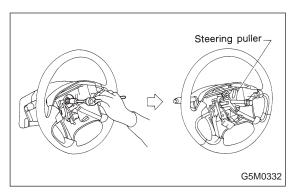
4) Remove steering wheel nut, then draw out steering wheel from shaft using steering puller.
