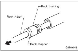
3) Pull rack assembly from cylinder side, and draw out rack bushing and rack stopper together with rack assembly.
