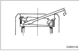
3) Pry off oil seal using screwdriver.
