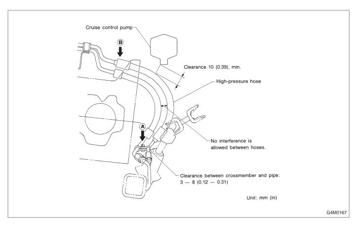
11) Finally check clearance between pipes and/or hoses, as shown above.
