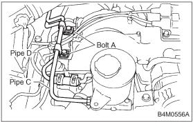
5) Disconnect pipe C·D from pipe (on the gearbox side). **CAUTION:**
