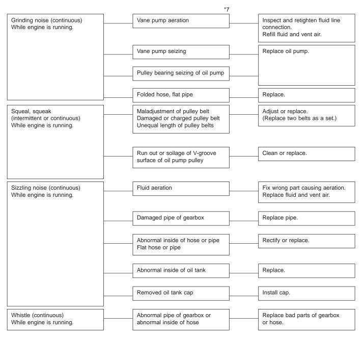
\*7 Grinding noise may be heard immediately after the engine start in extremely cold condition. In this case, if the noise goes off during warm-up there is no abnormal function in the system. This is due to the fluid characteristic in extremely cold condition.
