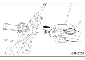
Sliding resistance: Right-turn steering 304 N (31 kg, 68 lb) or less Left-turn steering 304 N (31 kg, 68 lb) or less
