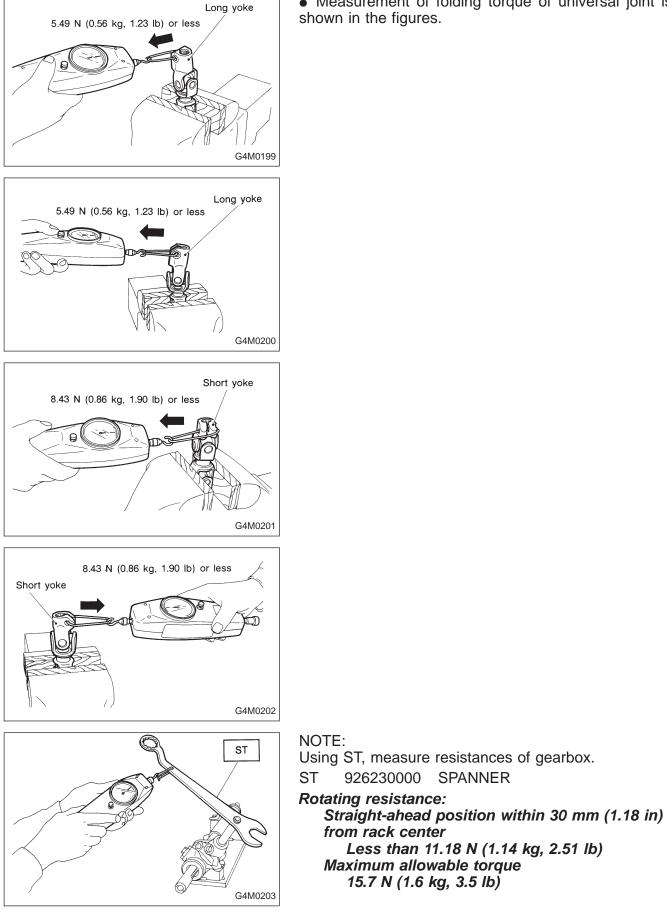
• Measurement of folding torque of universal joint is as shown in the figures.
