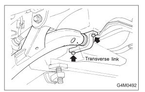
3) Remove nut (do not remove bolt.) securing transverse link to crossmember.
