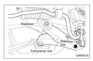
3) Remove bolts which secure stabilizer link to front transverse link.
