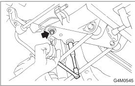
6) Remove bolts securing crossmember to vehicle body, and remove crossmember.
