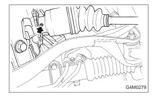
2) Install DOJ on transmission spindle and drive spring pin into place.
