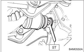
3) Insert DOJ spline end into bore of side oil seal, and remove ST.
