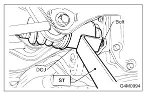
8) Remove DOJ from rear differential using ST. ST 28099PA100 DRIVE SHAFT REMOVER NOTE:
