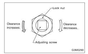
Adjustment of the adjusting screw
