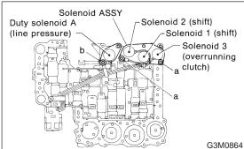
(6) Remove control valve body and two brackets. Remove 6 long bolts (Black) and 11 short bolts (Yellow).NOTE:
