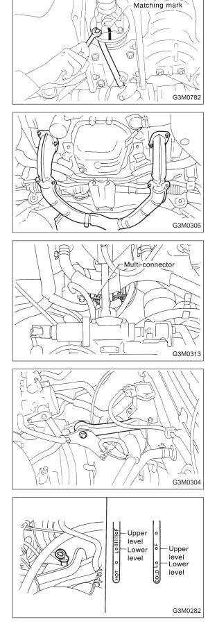
(5) Install propeller shaft.
