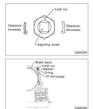
2) In case of the occurrence of problems 1. and 4. mentioned previously, perform the adjustment as follows: Adjusting procedure: Tighten adjust screw to 9 N·m (0.9 kg-m, 6.5 ft-lb) torque, then back off three turns.
