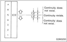
(4) Check if there is continuity at equal points when the select lever is turned 1.5° in both directions from the N range.
