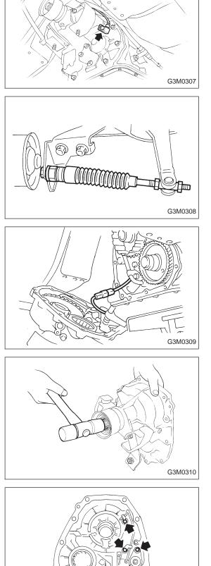
(6) Remove vehicle speed sensor 1.
