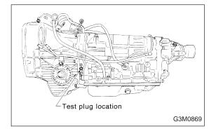
1) Line pressure measurement (under no load)
