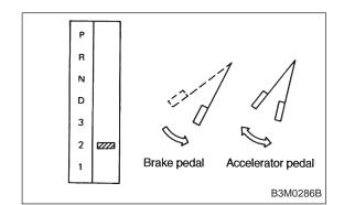
Be sure to cool down the engine for at least one minute after each stall test with the select lever set in the P or N range and with the idle speed lower than 1,200 rpm. If the stall speed is higher than the specified range, attempt to finish the stall test in as short a time as possible, in order to prevent the automatic transmission from sustaining damage.
