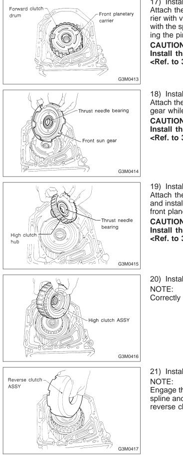
17) Install the front planetary carrier.
