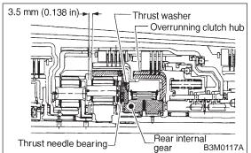
13) Install the one-way clutch outer race.
