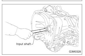
4) Extract the torque converter clutch assembly. NOTE:
