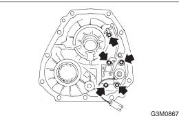
2) Remove duty solenoid C, transfer valve body and the transfer pipe.
