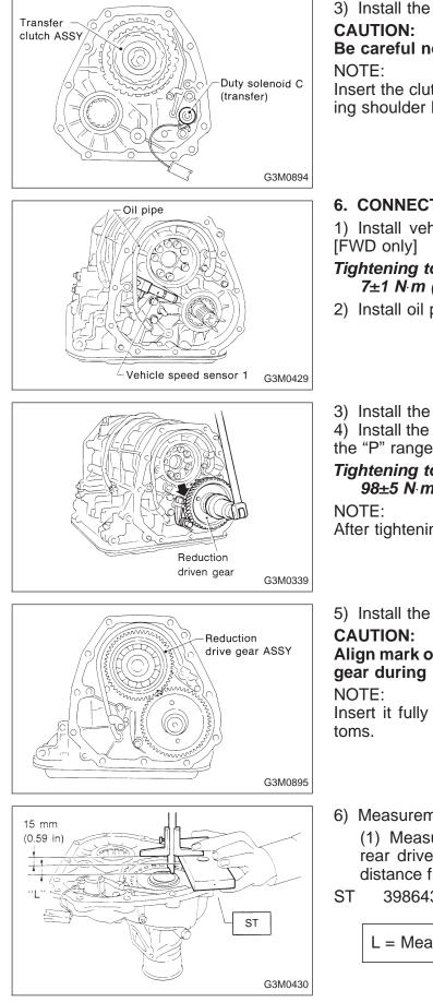
3) Install the transfer clutch assembly to the case.
