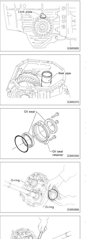
(9) If tooth contact is correct, mark the retainer position and loosen it. After fitting the O-ring, screw in the retainer to the marked position. Then tighten the lock plate to the specified torque.
