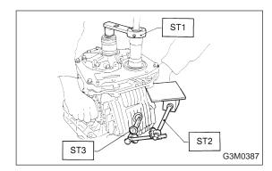
(7) Turn the drive pinion several rotations with ST1 and check to see if the backlash is within the standard value with ST2 and ST3.
