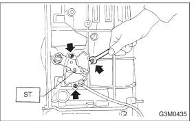
2) Installation and adjustment of inhibitor switch
