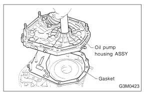
24) Install the oil pump housing assembly.
