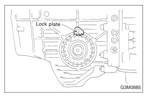
(2) Tighten four bolts to secure the roller bearing.
