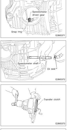
5) Remove the snap ring. Then remove the speedometer driven gear.
