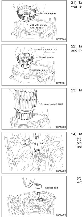
21) Take out the one-way clutch outer race and the thrust washer.
