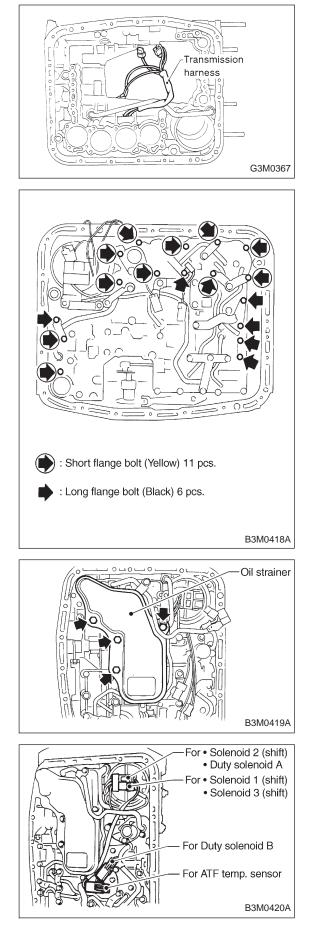
2) Install and route the transmission harness.CAUTION:Be careful not to damage the harness.
