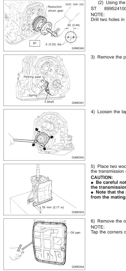
(2) Using the ST, extract the reduction driven gear.ST 899524100 PULLER SETNOTE:Drill two holes in the puller.
