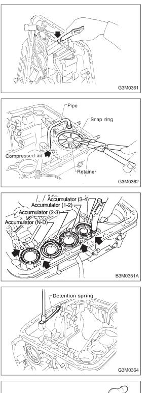
(3) Take out the low & reverse piston by applying compressed air.
