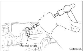
29) Remove the parking rod together with the manual lever. Then remove the manual shaft by pulling off the straight pin.
