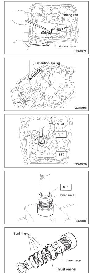
4) Assemble the manual lever and parking rod to the inside shaft, and secure with a nut.
