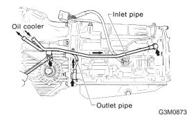
9) Remove the oil cooler inlet and outlet pipes. CAUTION:
