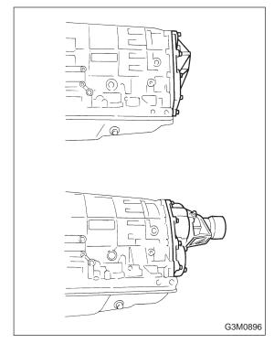
7) Installation of extension case (AWD), transmission cover (FWD) and transmission case.
