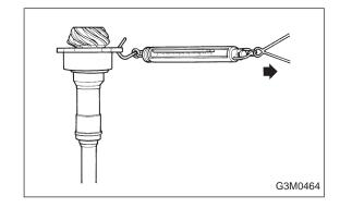
5) Measure the starting torque of the bearing. Make sure the starting torque is within the specified range. If out of the allowable range, replace the roller bearing.
