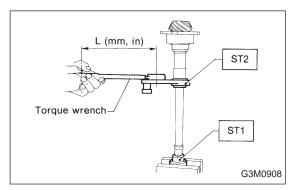
4) Tighten the lock washer and lock nut with ST1.
