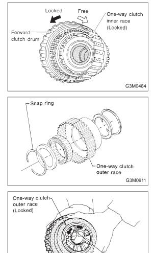
9) Install the one-way clutch (1-2) and plate, and secure with the snap ring.
