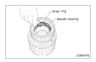
8) Install the needle bearing, and secure with the snap ring.
