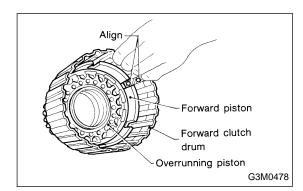
1) Fit the forward piston and overrunning piston to the forward clutch drum.
