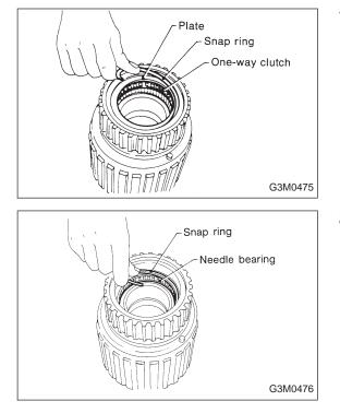
7) Remove the one-way clutch after taking out the snap ring.
