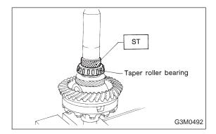
4) Measurement of backlash (Selection of washer) Measure the gear backlash with ST1 and ST2, and insert ST2 through the access window of the case.
