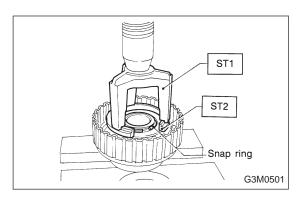
3) Install the driven plates, drive plates, and pressure plate, and secure with a snap ring with ST1, ST2 and a press.
