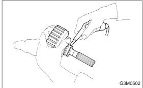
4) Apply compressed air to see if the assembled parts move smoothly.
