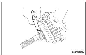
5) Apply compressed air to the rear drive shaft to remove the piston.
