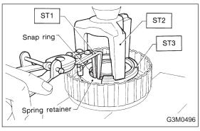
4) Remove the snap ring with ST1, ST2 and ST3, and take out the spring retainer.
