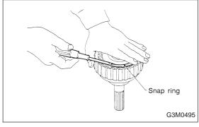
3) Remove the snap ring, and take out the pressure plate, drive plates, and driven plates.
