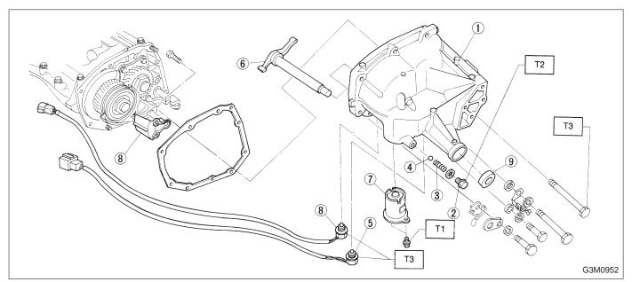
Tightening torque: N·m (kg-m, ft-lb) T1: 6.4±0.5 (0.65±0.05, 4.7±0.4) T2: 10±1 (1.0±0.1, 7.2±0.7) T3: 25±2 (2.5±0.2, 18.1±1.4)
