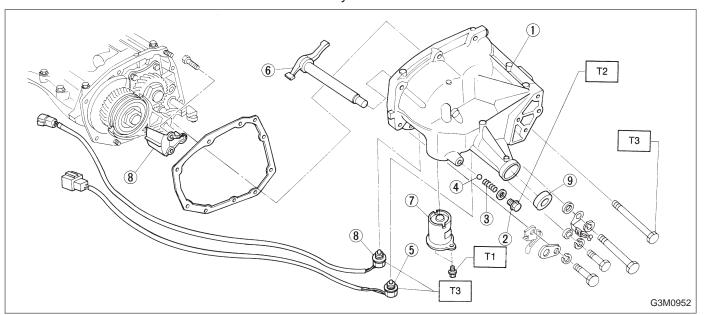
Tightening torque: N·m (kg-m, ft-lb) T1: 6.4±0.5 (0.65±0.05, 4.7±0.4) T2: 10±1 (1.0±0.1, 7.2±0.7) T3: 25±5 (2.5±0.5, 18.1±3.6)
