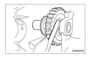
(2) After installing a suitable reverse shifter lever, shift into neutral. Using a thickness gauge, measure clearance between reverse idler gear and transmission case wall and adjust with washer(s).
