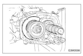
3) Remove main shaft rear plate 4.
