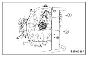
1) Remove clutch release lever 1 and bearing 2. (Refer to 2-10 clutch.)
