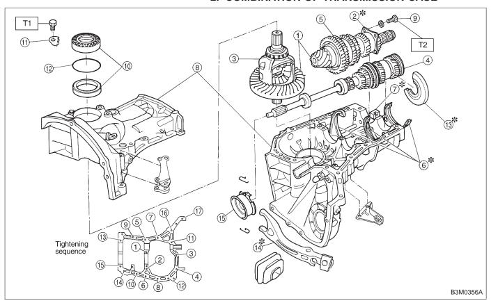
Tightening torque: N·m (kg-m, ft-lb) T1: 25 (2.5, 18)
