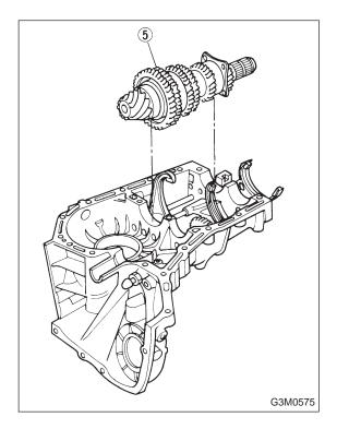
5) Install drive pinion shaft assembly (5) with shims selected before into transmission case.
