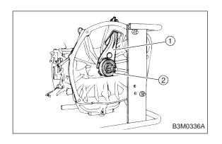
13) Install clutch release lever (1) and bearing (2).
