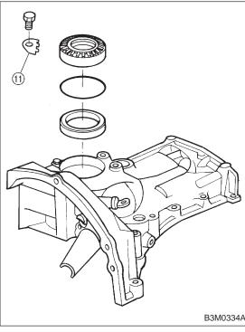
(4) Fit lock plate ①. Loosen the retainer on the lower side by 1-1/2 notches of lock plate and turn in the retainer on the upper side by the same amount in order to obtain the backlash.
