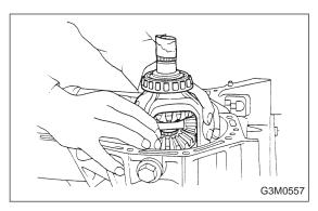
3) Install differential assembly ③ on left hand transmission case.
