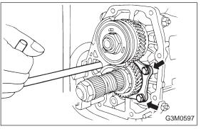
2) Remove bearing mounting bolts.
