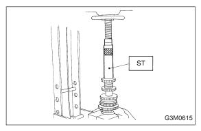
3) Install 2nd driven gear, 1st-2nd baulk ring and insert onto driven shaft. After installing key on driven shaft, install 3rd-4th driven gear using ST and press.
