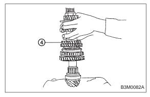
2) Install thrust bearing (33 x 50 x 3) and needle bearing (30 x 37 x 23). Install driven shaft assembly (4).
