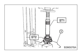
1) Install 1st driven gear, 1st-2nd baulk ring and gear and hub assembly onto driven shaft.
