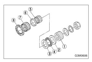
4) If starting torque is not within specified limit, select new adjusting washer No. 1 2 and recheck starting torque.
