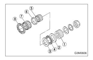
5) If specified starting torque range cannot be obtained when a No. 1 ② adjusting washer is used, then select a suitable No. 2 ③ adjusting washer from those listed in the following table. Repeat steps 1) through 4) to adjust starting torque.
