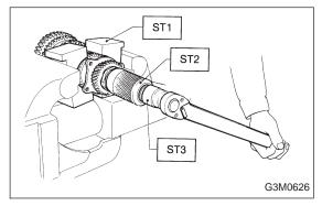
2) Using ST1, ST2 and ST3, tighten lock nut to the specified torque.
