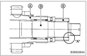
3) Install drive pinion collar 5, needle bearing 6 (25 x 30 x 20), adjusting washer No. 2 7 (25 x 36 x 4), thrust bearing 8 (25 x 37.5 x 3), adjusting washer No. 1 9 (25 x 36 x t) and differential bevel gear sleeve 1 in that order.
