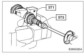
3) After removing ST2, measure starting torque using torque driver.
