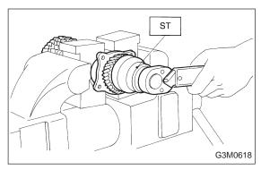
6) Install lock washer (42 x 53 x 2). Install lock nut (42 x 13) and tighten to the specified torque using ST.
