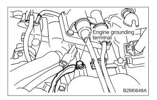
7) Use engine grounding terminal or engine proper as the grounding point to the body when measuring voltage and resistance in the engine compartment.
