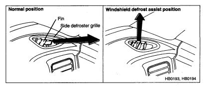
The driver's side defroster grille is adjustable. The normal positions as shown in the diagram directs warm air to the side glass. When more rapid defrosting of the windshield is desired, the air flow can be directed temporarily toward the windshield to assist the windshield defroster. If this is done, the driver's side grille should always be returned to its normal positions so that the warm air flow can then be used to defrost the driver's side window.
