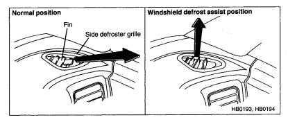
The driver's side defroster grille is adjustable. The normal positions as shown in the diagram directs warm air to the side glass. When more rapid defrosting of the windshield is desired, the air flow can be
