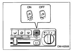
**ON position:** Interior air is recirculated inside the vehicle. Push the air inlet selection button to the ON position. The indicator light will come on. **OFF position:** Outside air is drawn into the passenger compartment. Push the air inlet selection button again to the OFF position. The indicator light will go off.
