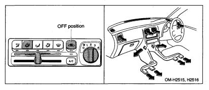
To direct air of different temperatures from the instrument panel outlets and foot outlets. The cool air will flow from the instrument panel outlets and warm air flows from the foot outlets.
