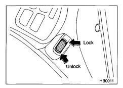
All doors and the rear gate (for wagon) can be locked and unlocked by the power door locking switches at the driver's side and the front passenger's side doors.
