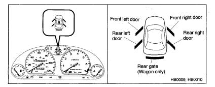
Your vehicle is equipped with door open warning lights. When a door is not fully closed, a light comes on indicating specifically which door it is. When all doors are properly closed, all of the door open warning lights go out. Always make sure these lights are out before starting to drive.
